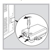
screwdriver into the side tabs of the cover. Use the screwdriver as a lever by pushing it down to open the cover (see diagram).
